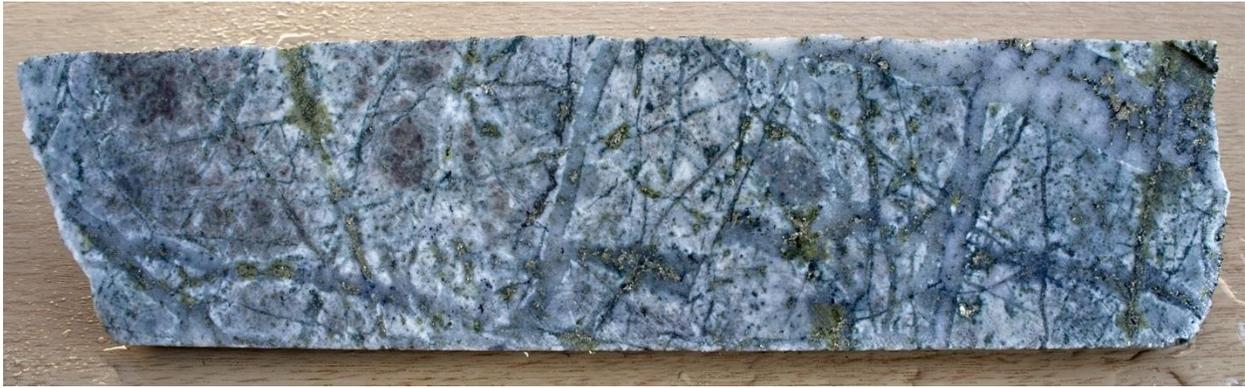
**Image 2.** ELID019, 246.2m from a sample interval reporting **2.62% Cu, 0.031% Mo, 21.8 g/t Ag**. Semi-massive chalcopyrite-pyrite associated with a 5 cm wide A-type quartz vein. Core is HQ diameter (63.5 mm).
